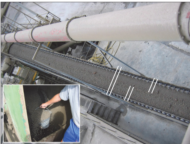
Figure 3. Examples of irregular, unacceptable, partial cross-section slices compared to a correct full slice of the moving stream; the first two do not comply with the definition of correct increments. Observe also the marked asymmetrical load on the conveyor belt, which would wreak havoc with either of the partial cross-sections. The insert shows when this adverse issue is taken to its extreme, with no observance of the need of securing a balanced cross-section of the moving stream. Indeed, here the objective here seems to be “get a full bucket with the least hassle”, which does not make for representativity—it is grab sampling plain and simple. Photo credit: KHEC teaching collection.
