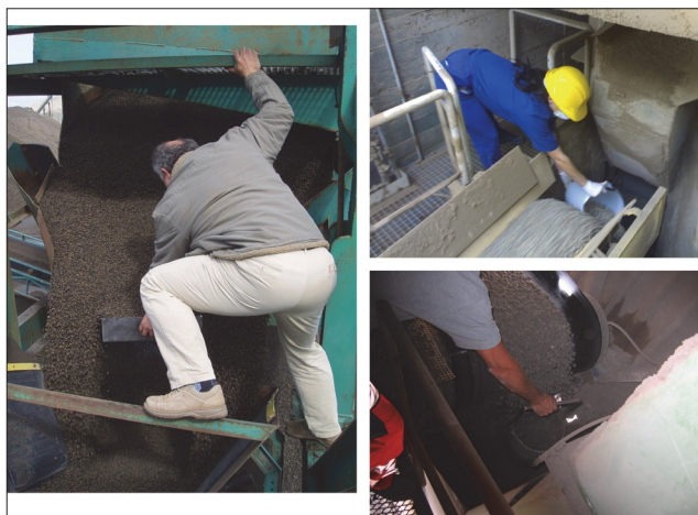
Figure 7. Horrific examples of extremely unbalanced, IDE/IEE-ridden attempts of manual increment process sampling—always doomed to fail. Manual process sampling is pretty much always a fatal give in to practical complacency. Photo credit: KHEC teaching collection.
