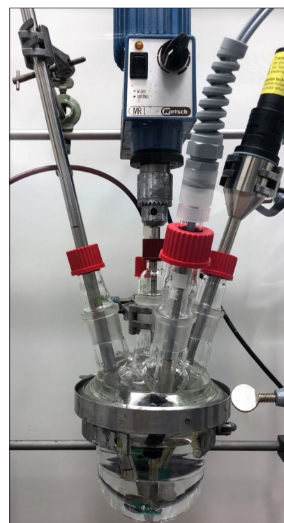
Figure 1. The setup used at the Open Days with the three probes inserted from above for simultaneous monitoring of the reagent being dosed from the rear port.
