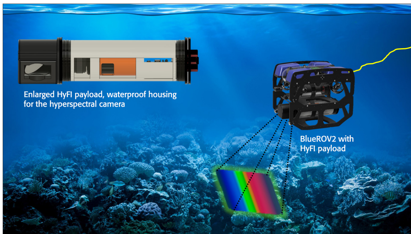
Figure 4. The hyperspectral fluorescence imaging (HyFI) payload, mounted on BlueROV2. Imaging around 1 m above the reef will provide an impact free rapid health assessment. The camera is housed in a custom waterproof housing with a 90° mirrored lens to allow for perpendicular imaging of the reef.
