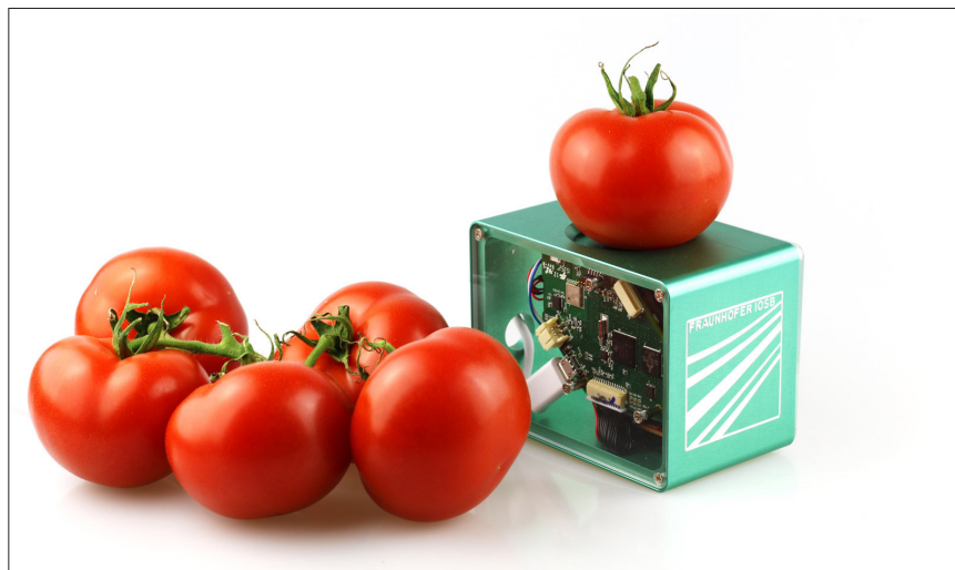
A compact food scanner based on NIR spectroscopy will help avoid unnecessary food waste. © Fraunhofer IOSB
