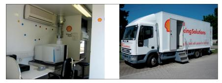
**Figure 1.** Left: Mobile ICP-OES instrument housed inside Racing Support vehicle; Right: Racing Support vehicle at Le Mans 24 hour race.
