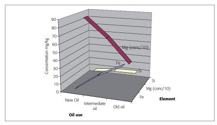
Figure 4. The elemental composition of the oil tested vs time.
