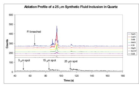
**Figure 2.** ICP-MS signal from ablation of a synthetic fluid inclusion, c.  $25\,\mu$ m in diameter. In this example the inclusion was first breached using a very small ( $5\,\mu$ m) laser spot, but there was no significant signal until it was fully opened with a  $15\,\mu$ m laser spot. This ablation removed the bulk of the contents, although the signal is irregular, and further ablation with a  $25\,\mu$ m spot removed a small amount of additional salts.
