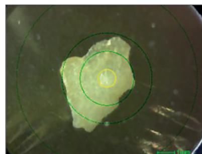
Figure 4. Photograph of contaminant (the yellow circle is the x-ray irradiation range: 1 mm Ø).
