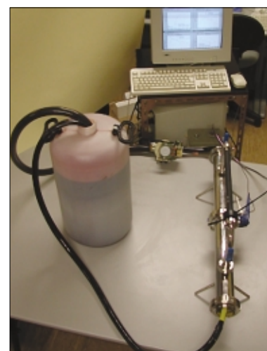
Figure 4. Closed circuit for calibration of sensor.
