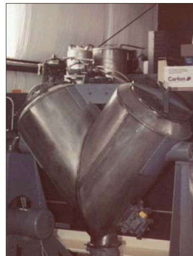
Figure 2. Crossfire "V" blender used to homogenise powders. This machine stands 2 m high and 3 m long. It can hold 250 kg of material.
