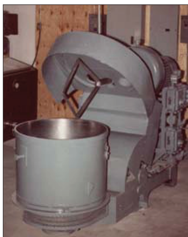
Figure 1. Annular change can heavy duty mixer used for soils and sediments prior to homogenisation.
