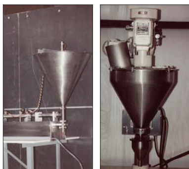
Figure 3. Variable stroke and bore filler for sludges and liquids (left) and filler for dry flowable and non-flowable materials.
