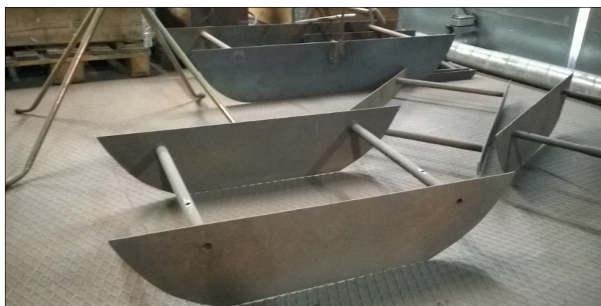
Figure 2. Example of a “stopped belt” sampling frame allowing a complete cross-section of the ore stream to be extracted. This will serve as a reference to the online sampling system (Figure 1). Image credit: LKAB.
