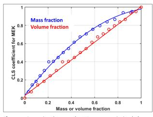
**Figure 1.** Comparison between the NIR spectroscopic signal of a binary mixture of chloroform/MEK (methyl ethyl ketone).
