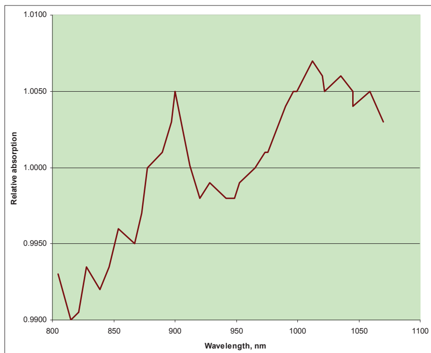
Figure 4. Output readings after division by the average value of the 11 readings for the appropriate tuning wheel position.
